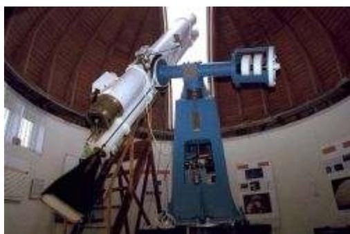
Vic then took us to the McClean dome, which houses the even larger McClean telescope (left). This is also a refracting telescope (collecting light with a lens). The lens is a foot wide, compared with the Kensington's ten inches. The telescope was originally commissioned by Frank McClean, a wealthy entrepreneur and keen amateur astronomer. His son Francis McClean supported Norman Lockyer in building his observatory at Salcombe Hill in 1912, and donated the telescope.
